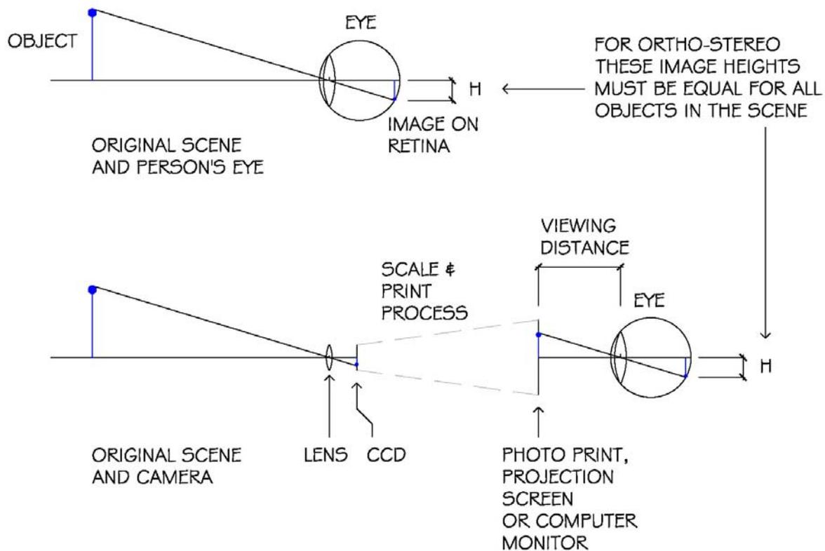
Fig 1 – Perspective requirements for ortho-stereo
