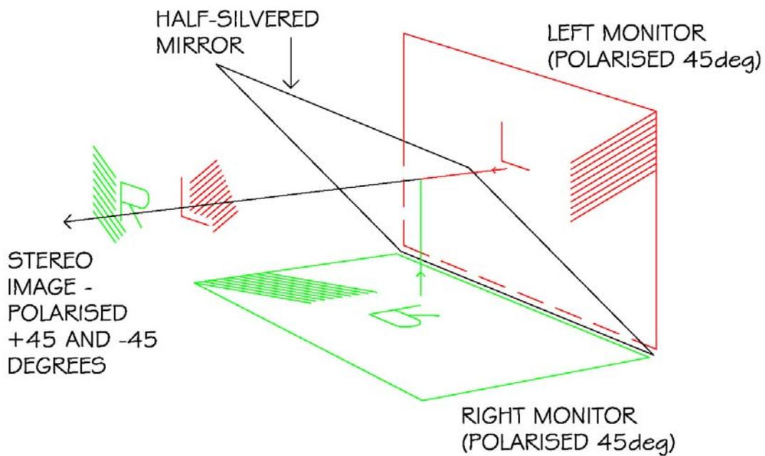
Fig 3 – Possible layout for polarised computer monitors. Note that the polarisation on each individual screen is the same orientation, but the mirror system results in orthogonal polarisation when viewed.
