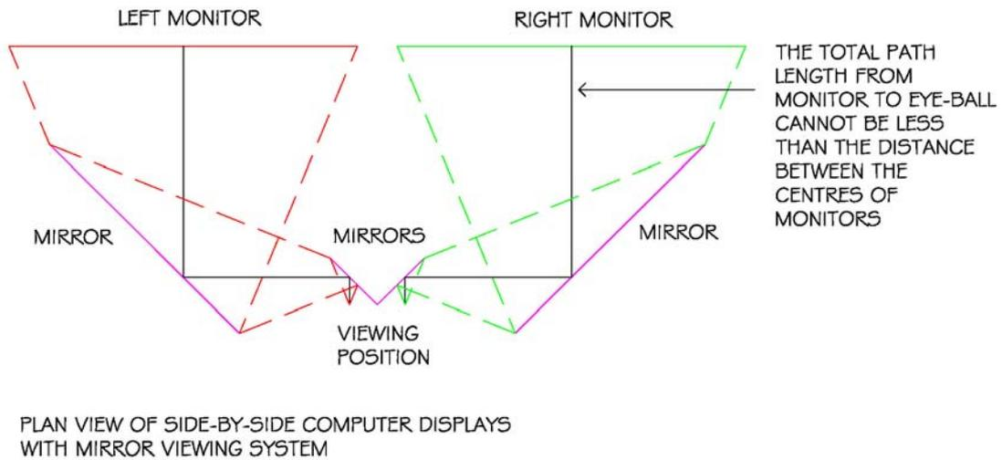
Fig 2 – Possible layout for side-by-side computer monitors and first-surface mirror system.
